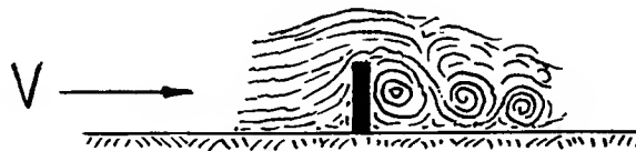
Figure 55. Flow pattern past a bluff obstacle (showing an alternating vortex street), traced from one of Leonardo da Vinci's drawings. — "Del Moto e Misura dell'Acqua", edited by Carusi and Favaro, Bologna 1923.
